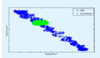
Thrust-Towing-force samples of one run by the Quasi-steady method versus the Conventional method
